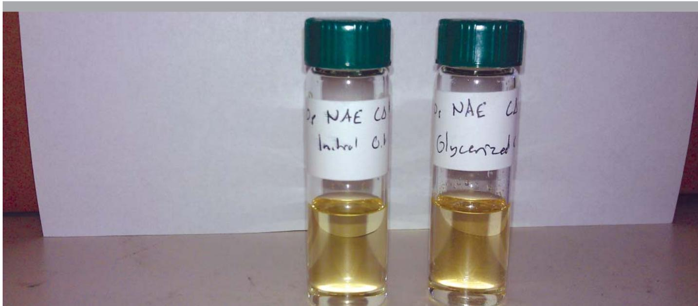
CLEAR AS DAY: Done under the right technique, oil produced via glycerolysis, right, results in a color nearly identical to feed oil, left.
